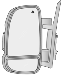
Warning Light Location
