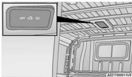
Ceiling Cargo Lamp
