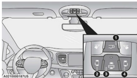
Overhead Console Power Switches
