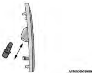
Front Side Marker Lamp Bulb Removal
