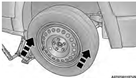
Mounting Inflatable Spare Tire
