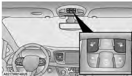
Courtesy Light Switches
