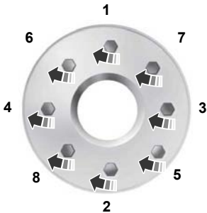
8-wheel nut torque sequence
