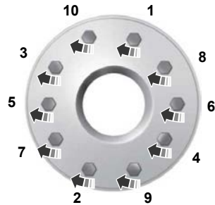
10-wheel nut torque sequence
