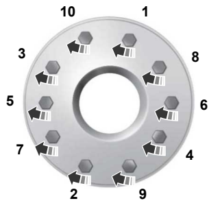
10-lug nut torque sequence.
