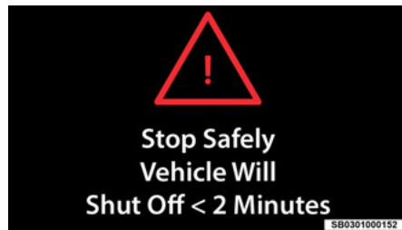
Stop Safely Vehicle Will Shut Off In Less Than Two Minutes Message
