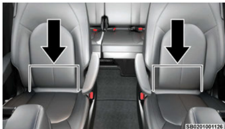
LATCH Anchorages (Second Row Anchorages Shown) Seven Passenger Quad and Stow 'n Go Seating
