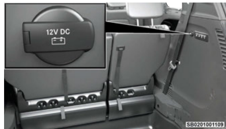
Rear Power Outlet
