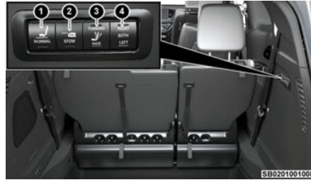
Rear Panel Power Switch Bank
