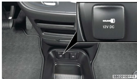
12 Volt Front Power Outlet (In Floor Tray) - If Equipped
