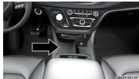
Wireless Charging Pad Location
