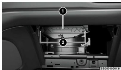
Fresh Air Inlet
