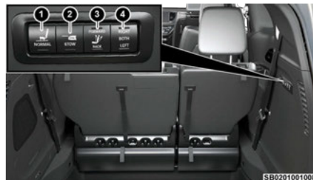
Rear Panel Power Switch Bank
