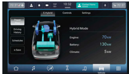
Power Flow Screen
