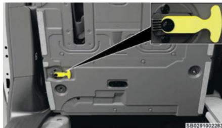
Storage Bin Cover Emergency Release Lever
