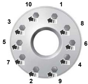
10-wheel nut torque sequence
